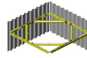
Steel Sheeting and Bracing
